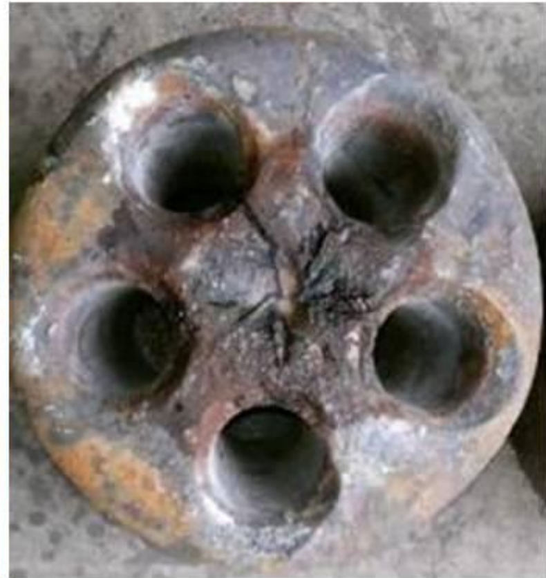
b) Cartridge tip face and damage due bad heat transfer
